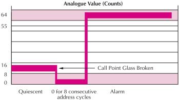
Fig.16 Typical response characteristic - XP95 Manual Call Point
